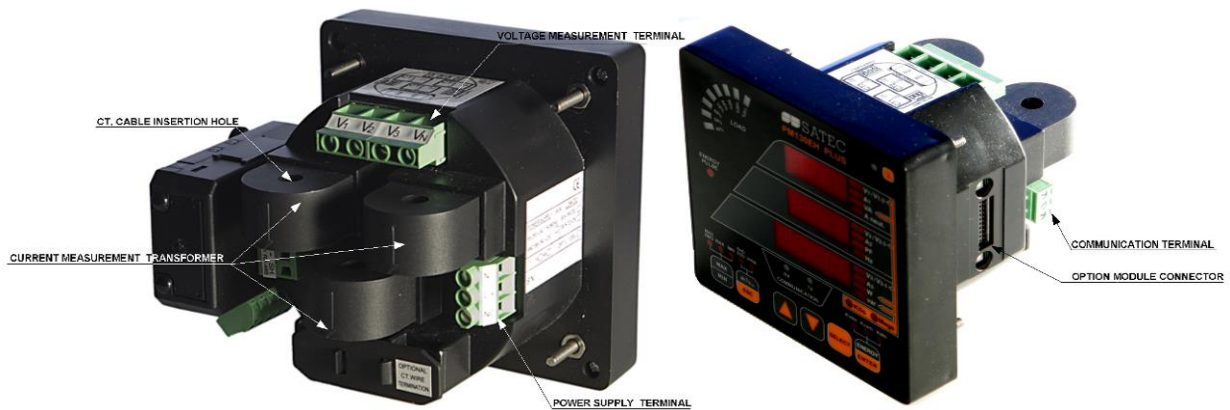
Figure 2-7 Terminals - Rear View
